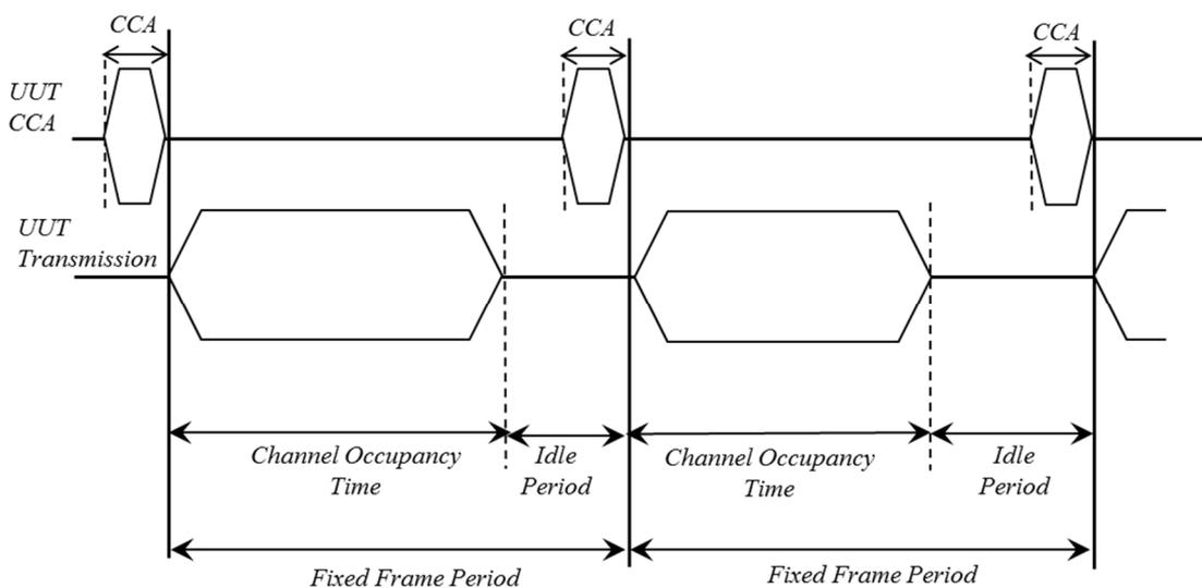
Figure 2: Example of timing for Frame Based Equipment
