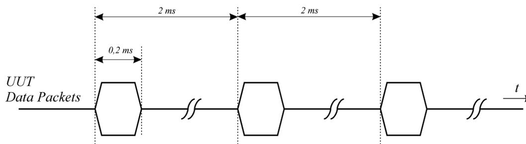
Figure 4: General structure of the test transmission sequences
