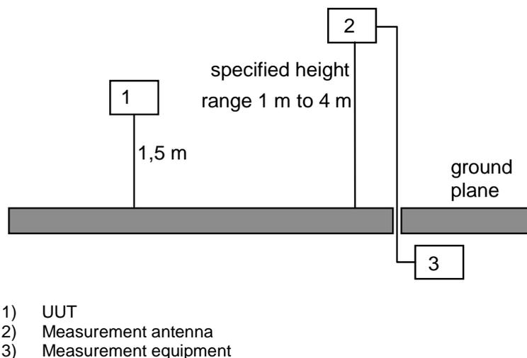
**Figure C.1: Measurement arrangement**
