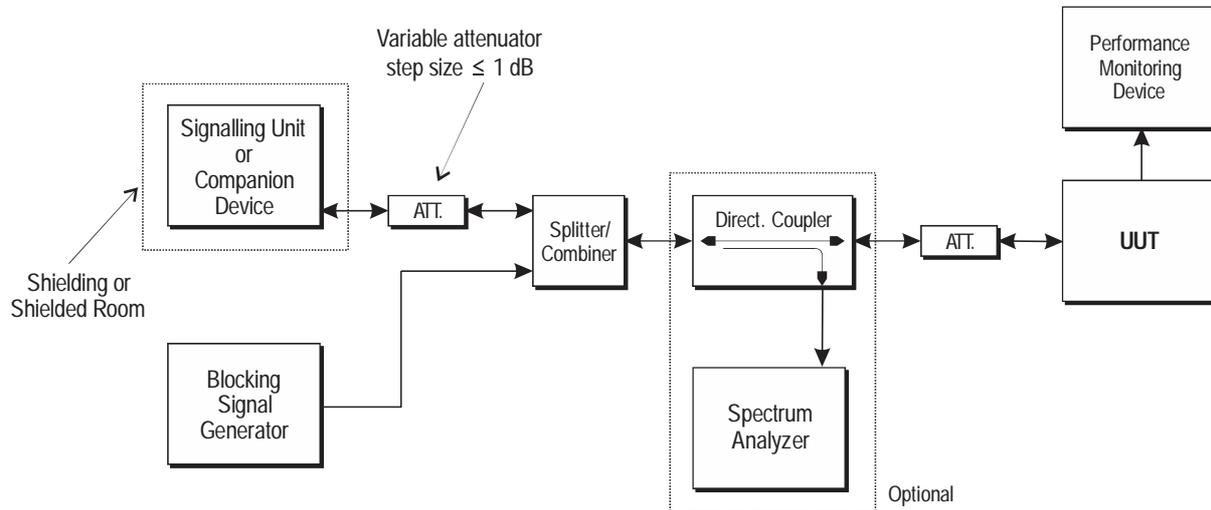
**Figure 18: Test Set-up for receiver blocking**
